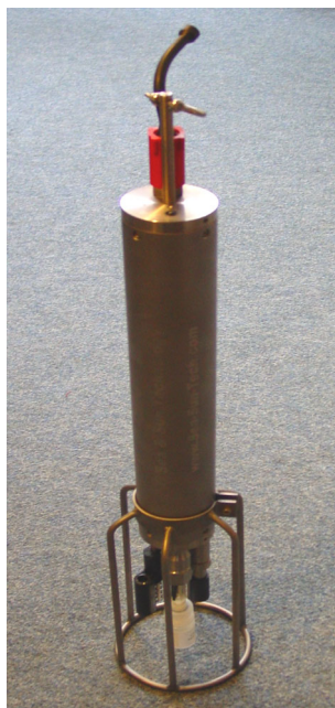
Abbildung 3: Multiparametersonde CT 161 (Sea & Sun Technology)
